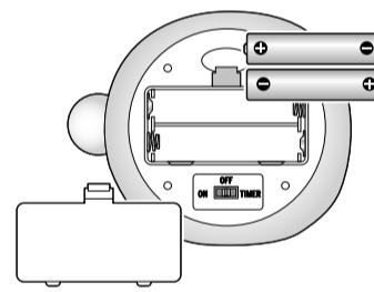
1. Remove the battery compartment lid.
